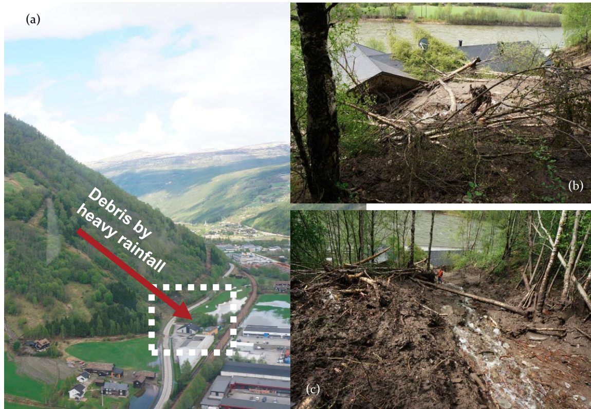
Figure 3. Debris flow occurrences on the example site: (a) general view of the impacted area and details of the debris flow impact on: (b) buildings and (c) vegetation.
