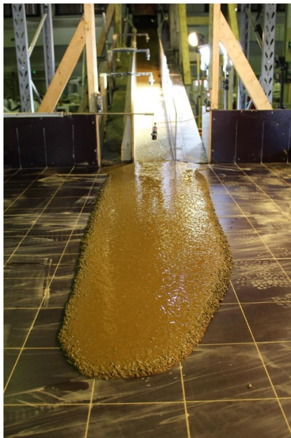
Figure 33: elongated deposit shape for test G2V1C1R1, with the front in detail
