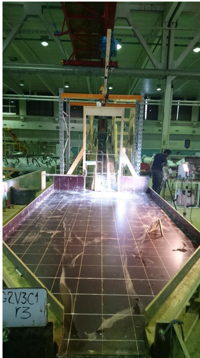
Figure 14: the physical model to test debris flows
