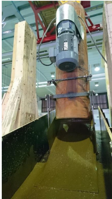
Figure 17: release cylinder. The cylinder contains a rotating device which allows to mix the debris material
