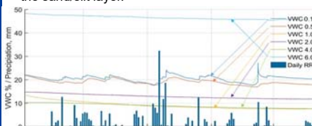
Figure 6: Volumetric water content and daily rainfall, Jun-Oct 2016
