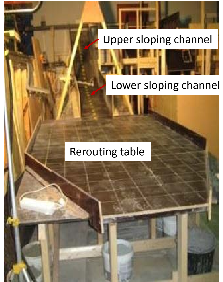
Model setup in the lab (Source: Christiansen, 2013)
