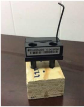
Figure 1 Omnisense sensor placed in an LVL sample, with the electrodes perpendicular to the grain direction. Also parallel to the grain direction was tested. The nails are not insulated.
